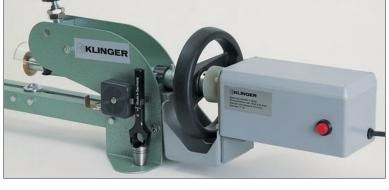
The electric drive motor is then to be attached by means of sliding the internally toothed plastic coupling onto the toothed pinion, so that the holder arm grips around the shaft drive of the circular slitter saw from below.
